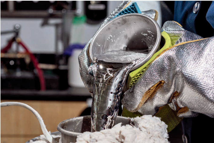
Associate Professor Asegun Henry is researching how to use hot metals like molten tin to store heat from a concentrated solar power system so it can be used to generate electricity as needed. Credit: Rob Felt, Georgia Tech
