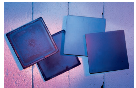
When placed under high temperatures and exposed to CO 2 , these ceramic membranes allow pure oxygen to pass through, leaving behind CO that can be used as fuel. Credit: John Freidah
