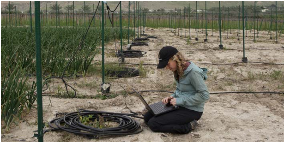
GEAR Lab researcher Carolyn Sheline troubleshoots a drip irrigation system at a full-scale test farm in the Jordan Valley where the team is piloting a low-cost precision irrigation controller that optimizes system energy and water use. Credit: John Freidah
