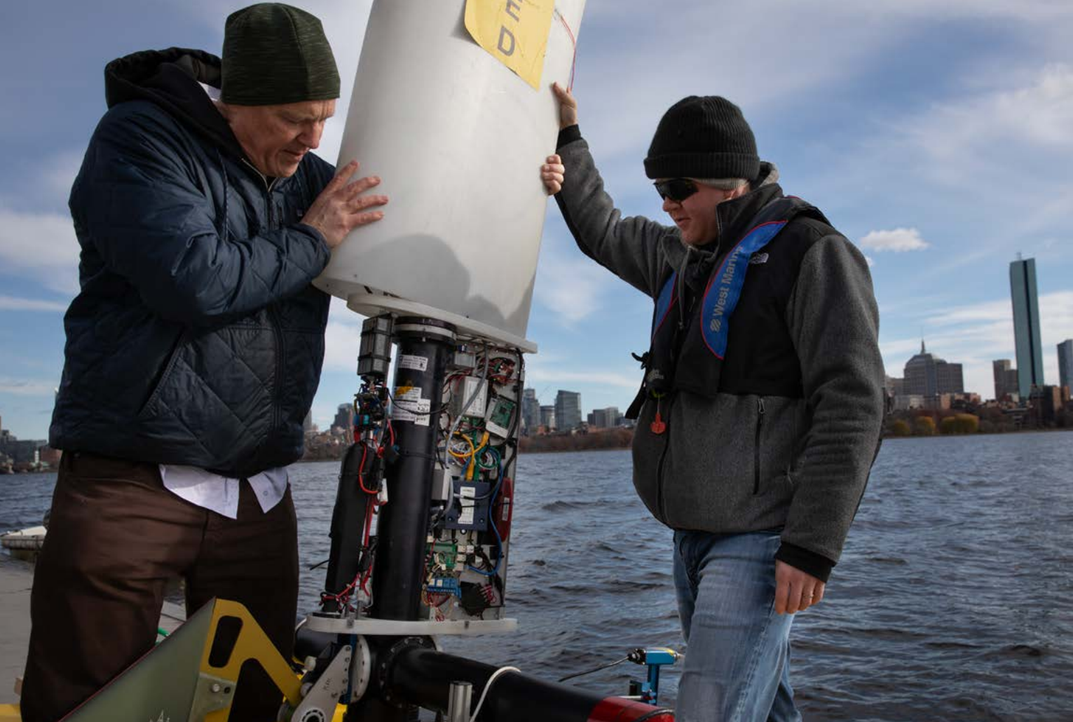
Principal Research Scientist Mike Benjamin, left, with MIT/WHOI Joint Program PhD student Tyler Paine, prepare the MIT autonomous sailboat for operations on the Charles River. The sailboat is manufactured by Marine Robotics, LLC, with MIT providing the autonomy software. Credit: John Freidah
