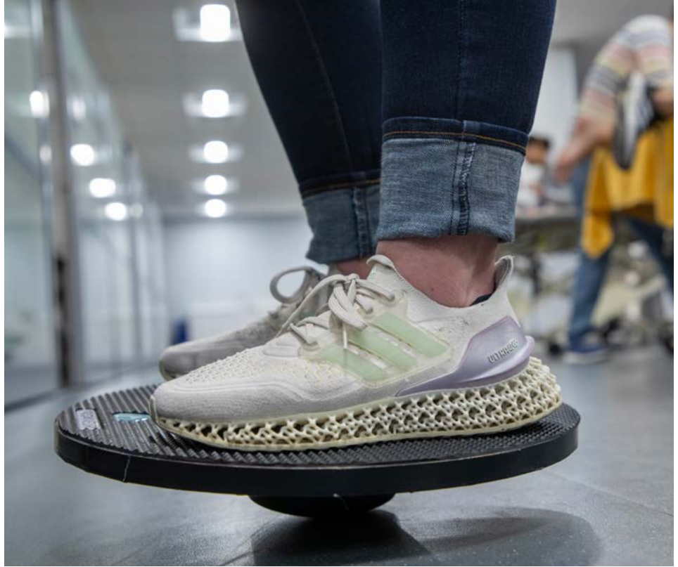
An instrumented balance board is used to gamify the recovery process for lower limb injuries and target the injuries' effects on the body's movement control systems. Credit: John Freidah
