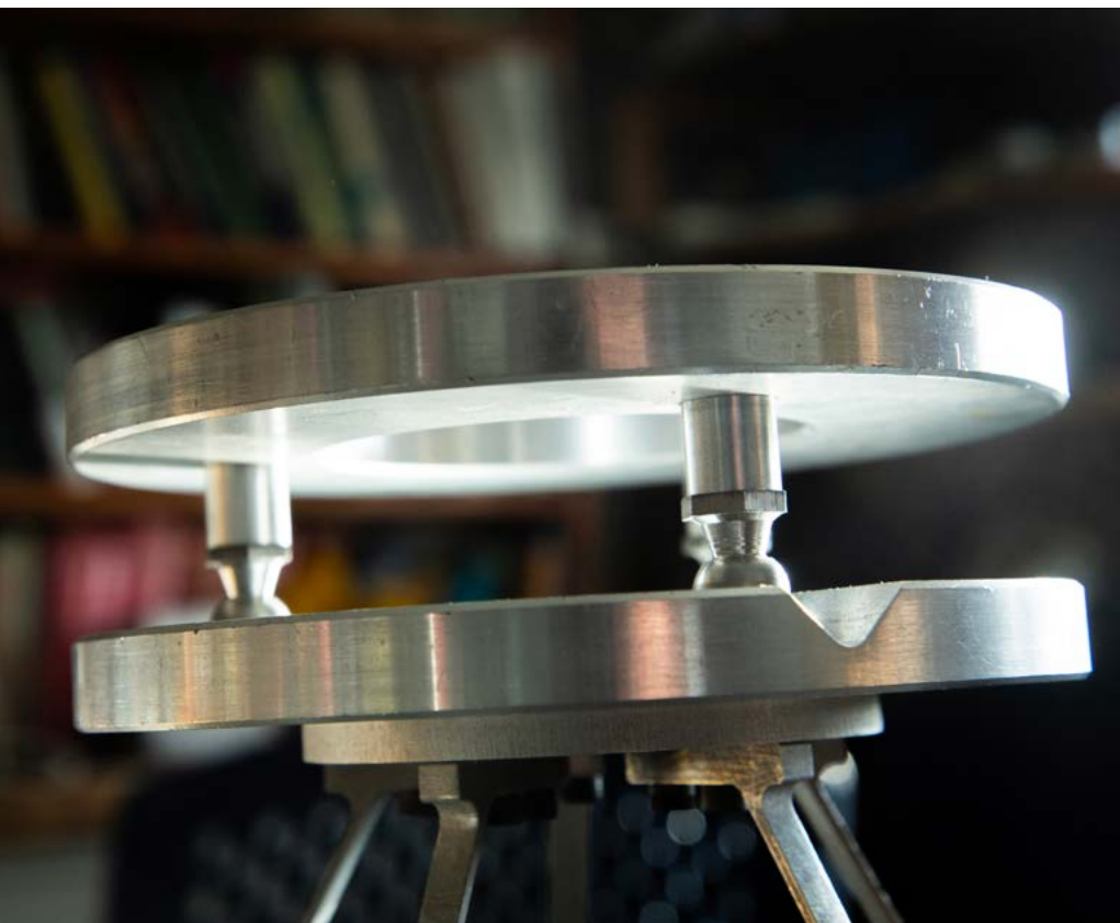
From Professor Alex Slocum’s lab, a kinematic coupling uses six points of unique, very stiff contact to establish the position and orientation between objects. Credit: John Freidah
