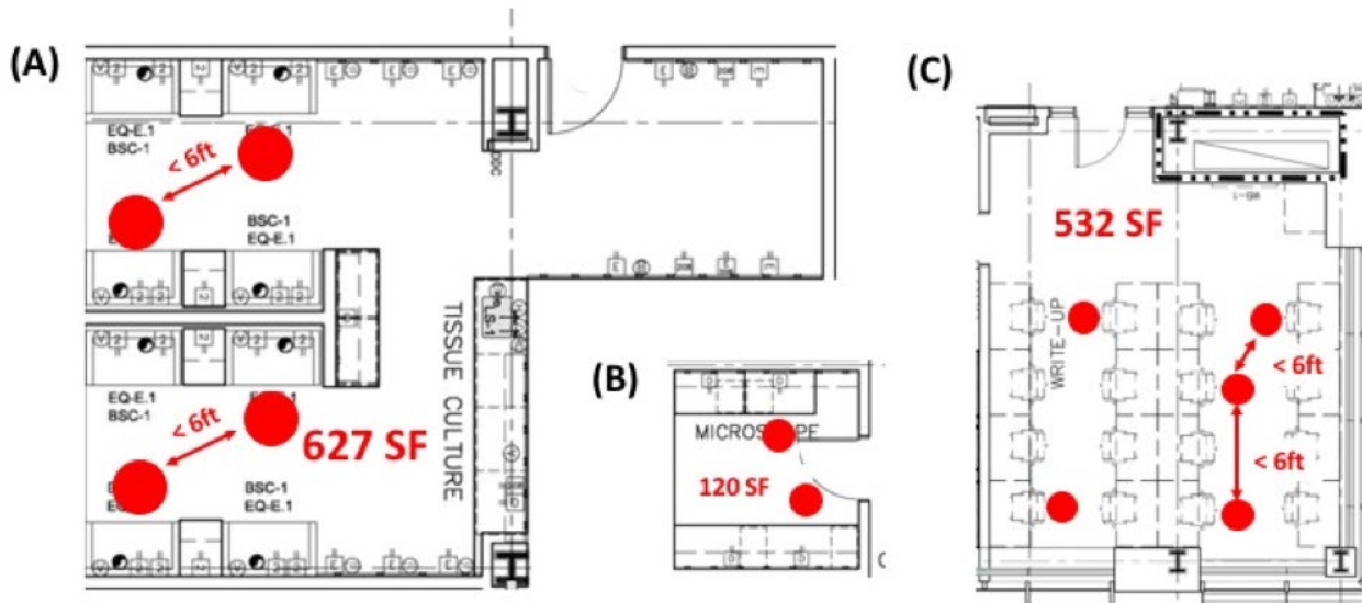
Figure 2. Examples of space plans that DO NOT meet the criteria for safe space layout. (A) A 627 sf tissue culture room can accommodate a maximum of 5 people working at static stations (solid circles); however, there needs to be 6 feet of physical distance between workers. (B) A 120 sf microscope room can only accommodate 1 person under the guidelines. (C) A 532 sf room can accommodate a maximum of 4 people, who must maintain 6 ft physical distancing.
